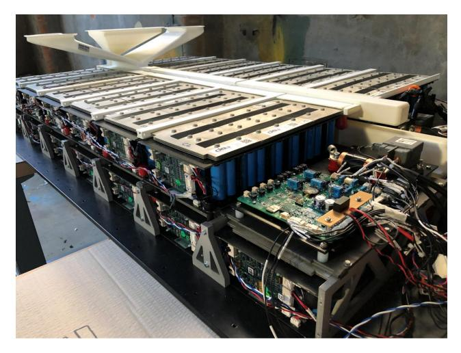
Industrial Modular Battery Pack Concept Addressing High Energy Density, Environmental Friendliness, Flexibility and Cost Efficiency for Automotive Applications
